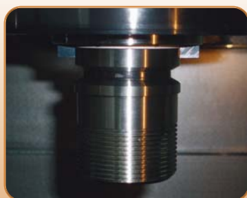
BT40 組立間隙量測-AA6061
